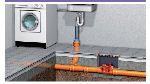
Staufix twin flap backwater valve - the classical item in the KESSEL backwater range and the successful original. The current model is made of ABS, completely corrosion-free and can be serviced without tools. Protects individual drainage fixtures such as shower, sink and washing machine below the backwater level. Installation in the concrete slab with upper section Art. # 32500 and two cover plates Art. # 30004 S or for installation in an exposed wastewater pipe.
