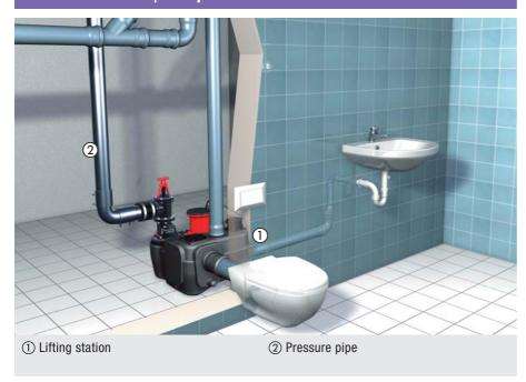
The lifting station Aqualift F is ideal for free-standing installation in frost-protected areas. The compact and powerful lifting station with control unit disposes of wastewater with or without sewage reliably and fully automatically through the pressure pipe to the higher-level sewage system.
