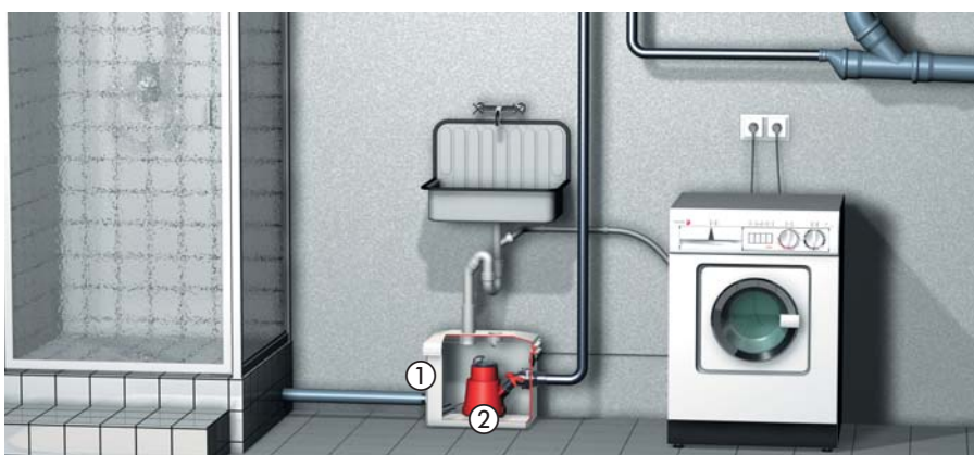
① Lifting station ② Wastewater pump
