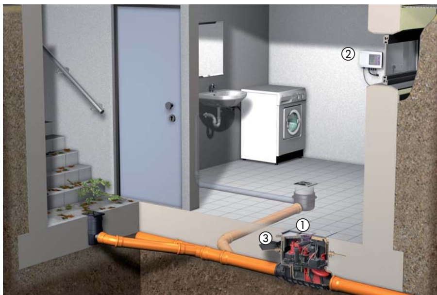
① Backwater pumping station ③ Sealing gasket set ② Control unit
