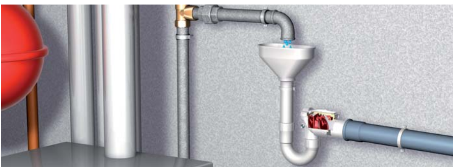
... furnace condensation overflow
