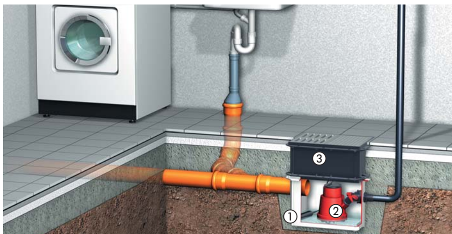
① Lifting station ② Wastewater pump ③ Extension section (Art. # 32 500)
